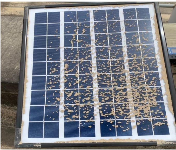
Figure 4.7 Coated panel after 24-hours
